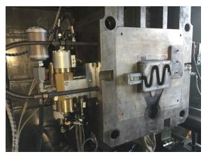
Lightweight design concepts are at the heart of the upcoming electric vehicle revolution. Forcing molten metals into a mould at high speed and pressure – high-pressure die casting – provides manufacturers with the flexibility to create complex components. Besides being lightweight, these are also strong and tolerant. The considerable increase in the use of light metal castings such as aluminium or magnesium presents a growth opportunity for the relevant industries.
